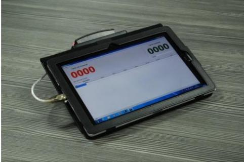
**Mobile Mustering Facility** – the PLAN software features a number of more conventional mustering features including the option to automatically print a roll-call list based on an evacuate signal from the fire system. Roll-call lists can also be emailed to off-site locations or printed in remote sites.
